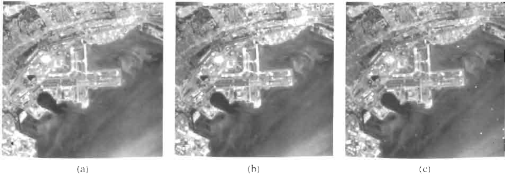
FIGURE 5 BTC with errors: (a) original image; (b) image compressed to 1.625 bpp; (c) performance of BTC in the presence of channel errors.
