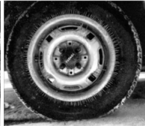
Tire after adaptive histogram equalization 8x8 tiles
