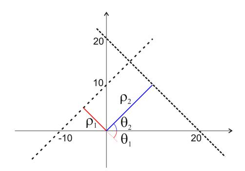
The Hough Transform will give two accumulation point for the sinusoids generated from the equation  $\rho = \overline{x} \cos \theta + \overline{y} \sin \theta$
