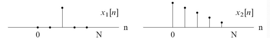
the circular convolution  $x_3[n] = x_1[n] \Re x_2[n]$  is the signal  $\tilde{x}[n]$  delayed by two samples, evaluated over the range 0 to N-1:
