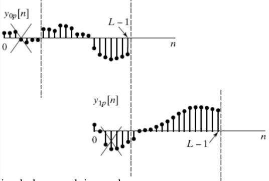
Result of circularly convolving each section with h[n]. The portions of each filter section to be discarded in forming the linear convolution are indicated
