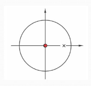
$$H_1(z) = \frac{1-\alpha}{1-\alpha z^{-1}} = z \frac{(1-\alpha)}{z-\alpha}$$
