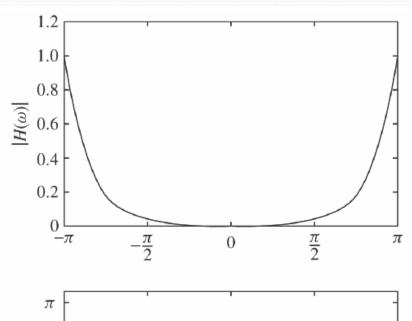
$$H_{2}(z) = \frac{1 - \alpha}{2} \frac{(1 - z^{-1})}{(1 + \alpha z^{-1})} = \frac{1 - \alpha}{2} \frac{(z - 1)}{(z + \alpha)}$$
