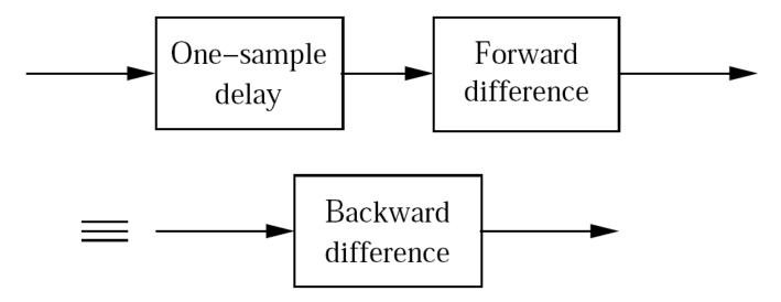
Here a non-causal system has been converted to a causal one by cascading with a delay. In general, *any non-causal FIR system can be made causal by cascading with a sufficiently long delay.*
