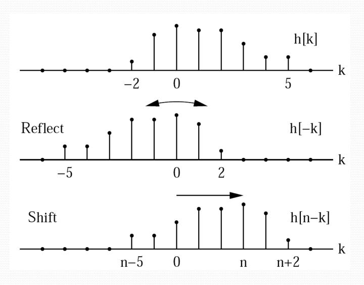
The sequence h[n-k] is then obtained by shifting the origin of the sequence to k=n.
