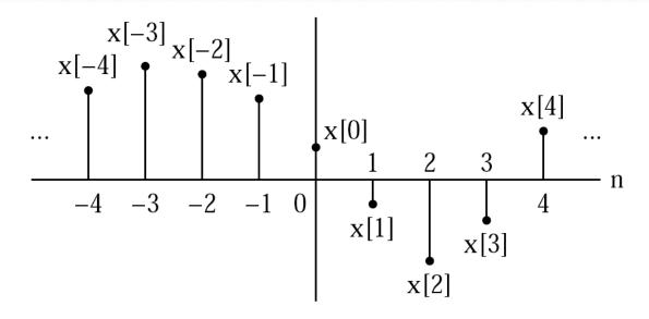
(This can be plotted using the MATLAB function stem.) The value x[n] is **undefined** for noninteger values of n.
