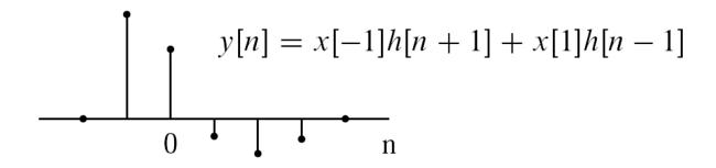
A slightly different interpretation, however, leads to a convenient computational form: the nth value of the output, namely y[n], is obtained by multiplying the input sequence (expressed as a function of k) by the sequence with values h[n-k], and then summing all the values of the products x[k]h[n-k]. The key to this method is in understanding how to form the sequence h[n-k] for all values of n of interest.
