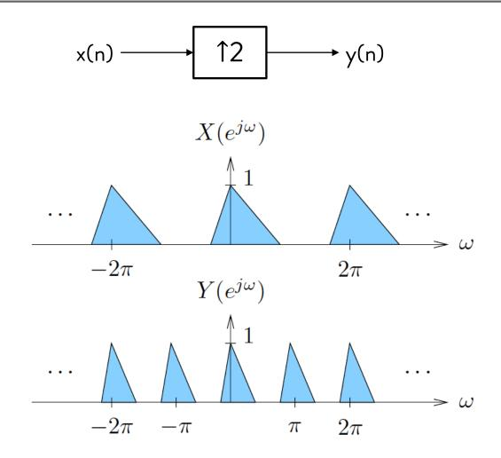
Spectral replicas do not overlap: upsampling just causes a compression of the spectrum, which has a new period of 1/L (or  $2\pi/L$ , or Fs/(L))
