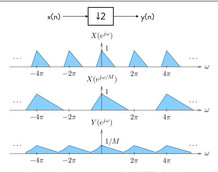
Aliasing in frequency occurs if the DTFT of x(n) is not limited to 1/(2M) (or  $\pi/M$ , or Fs/(2M))
