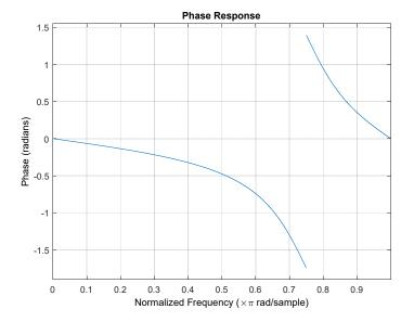
The jump of  $\pi$  degrees is clearly visible at the zero.
