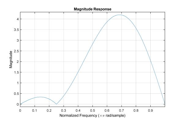
The sampled signal is  $x[n] = 3 + \cos\left(2\pi \frac{4\cdot 10^3}{16\cdot 10^3}n\right) + 3\cdot \sin\left(2\pi \frac{8\cdot 10^3}{16\cdot 10^3}n\right) = 3 + \cos\left(\frac{\pi}{2}n\right) + 3\cdot \sin\left(\pi n\right)$  and the filter will remove the continuous frequency and the sinusoid at the Nyquist frequency.
