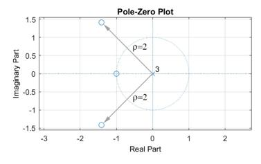
The two conjugate zeros are placed with an angle of  $\pm \frac{3}{4}\pi$  with respect to the positive real axis direction.
