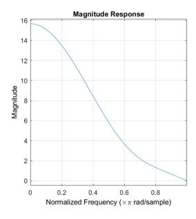
The component at the Nyquist frequency will be completely removed while the component at the  $\frac{\pi}{2}$  will be amplified by a factor of:  $\left|H_2\left(z=j\right)\right| = \left|4+\left(4+2\sqrt{2}\right)\left(-j\right)+\left(1+2\sqrt{2}\right)\left(-1\right)+j\right| = \sqrt{34} \simeq 5.83$
