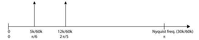
Normalized pulsations after downsampling: in red and green the spectral replicas of the signal due to downsampling. The aliased component is also indicated.
