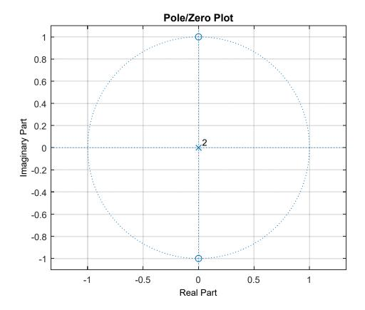
The component at 9kHz will also keep its amplitude since  $\left|H\left(z=e^{j\pi/4}\right)\right|=\left|H\left(z=e^{j3\pi/4}\right)\right|=1$
