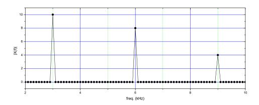
We sample the signal at 24 kHz and we want to build a filter H(z) to completely remove the carrier at 6kHz and keep unaltered the component at 3kHz.
